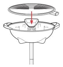
7. Position probe receptacle through probe cutout in top side of grill base.
